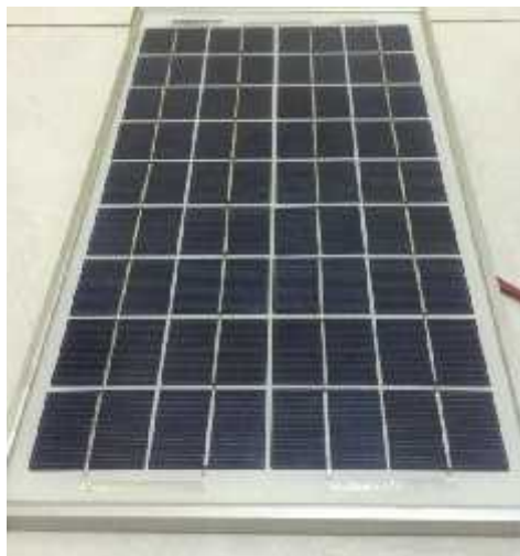
Gambar 4.2 Panel surya 10 Watt
